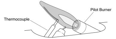
Figure 17 - Correct Pilot Flame Pattern
